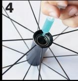
If necessary clean the bearing with a brush and some light degreaser. Re-grease the bearing. Mount the seal and the end-cap.
