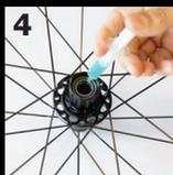
If necessary clean the bearing with a brush and some light degreaser. Re-grease the bearing. Mount the seal and the end-cap.
