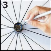
Gently remove the bearing seal with a narrow blade. Be careful not to cut the seal.
