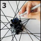
**3** Gently remove the bearing seal with a narrow blade. Be careful not to cut the seal.
