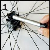
**1** Remove the disc brake allowing access to extract the axle.
