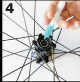
**4** If necessary clean the bearing with a brush and some light degreaser. Re-grease the bearing. Mount the seal and the end-cap. Replace the disc brake according to the manufacturers instructions.
