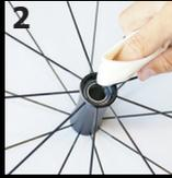
Wipe any dirt and contamination away from the bearing, hub and end-cap.
