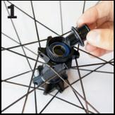
**1** Remove the disc brake allowing access to remove the end-caps.
