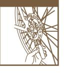
When your disc brake rotor is not centered and rubbing, combine the tool with a CO2 cartridge. CO2 cartridge can be used as a longer lever arm and easier to operate, and help adjust the problem of disc brake rubbing. During the process of adjusting the rotor, avoid over-adjusting in a single position.
